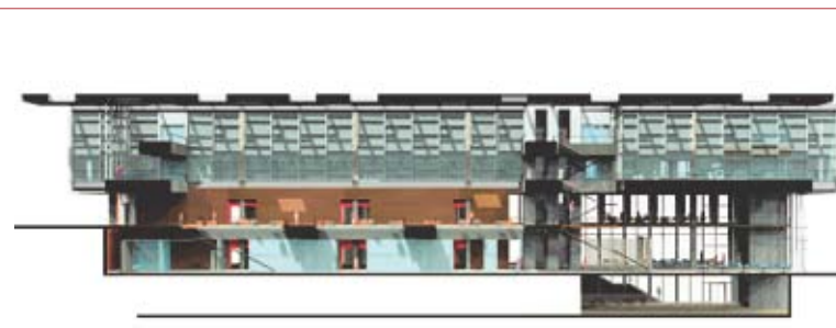
Section looking Northeast. Faculty offices are on the upper floors connected to the atrium through a series of bridges and stairs. Undergraduate and graduate student areas and classrooms are linked directly in to this central community space on the lower levels.
