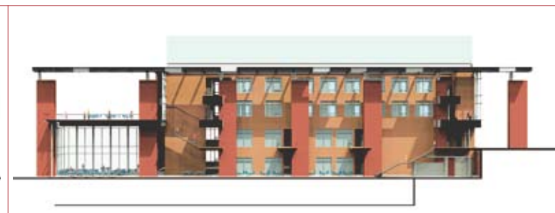
Section looking Southwest. Brick and wood are used extensively on the interior of the atrium. Combined with close attention to daylighting and acoustic requirements, this central community space will form an inviting environment for a broad array of student, staff, and faculty interactions. The café sitting area and covered outdoor terrace overlooking Denny Yard are on the left.
